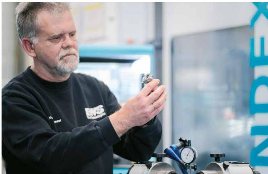
Left: The bevel gears that have just been machined are tested on a gear rolling tester machine alongside the INDEX G220.
