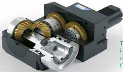
The bevel gears produced in-house are used in all EWS driven tools. (Photos: EWS)
