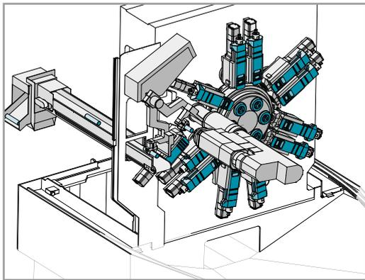
Position-aligned workpiece removal with integral parts conveyor
