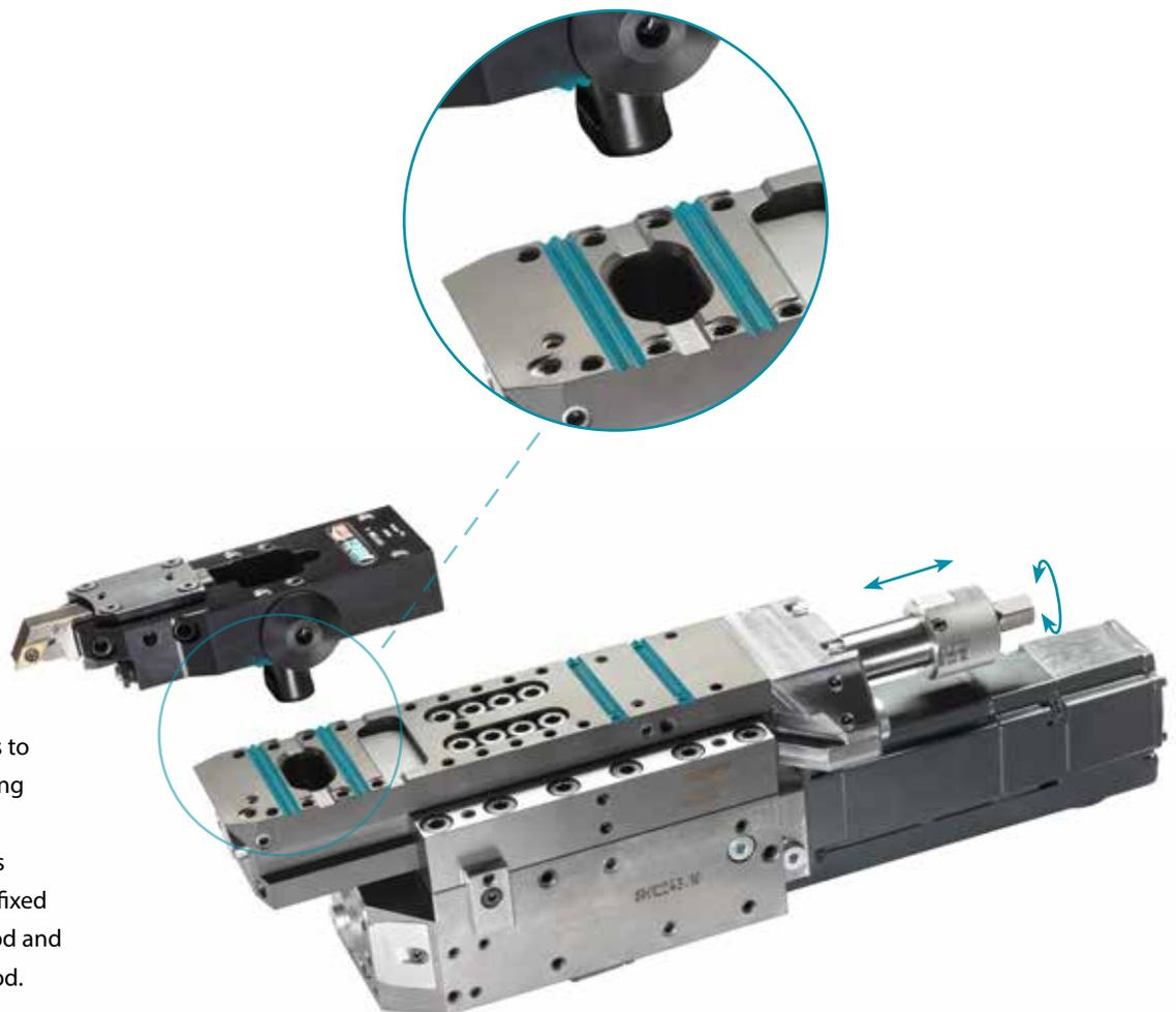
50% time-saving thanks to the INDEX quick clamping system with integrated W-serration on the cross slide: The tool holder is fixed in position using a tie rod and pre-tensioned wedge rod.
