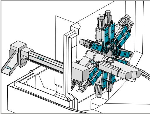
Stationary workpiece removal device with integral parts conveyor
