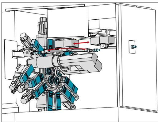
Position-aligned workpiece removal with intermediate gripper and linear shuttle
