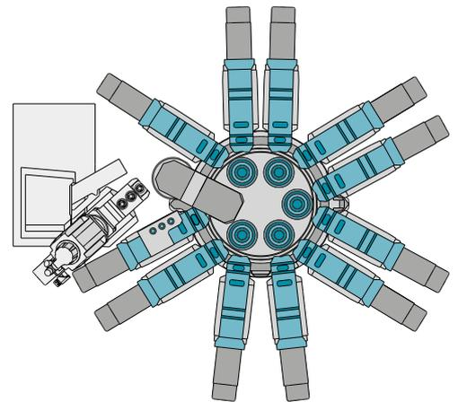
The double three-spindle machine – for maximum work output
