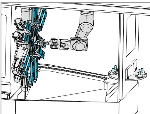
Parts feed and removal by a 6-axis robot via the swivel disk to the external handling system
